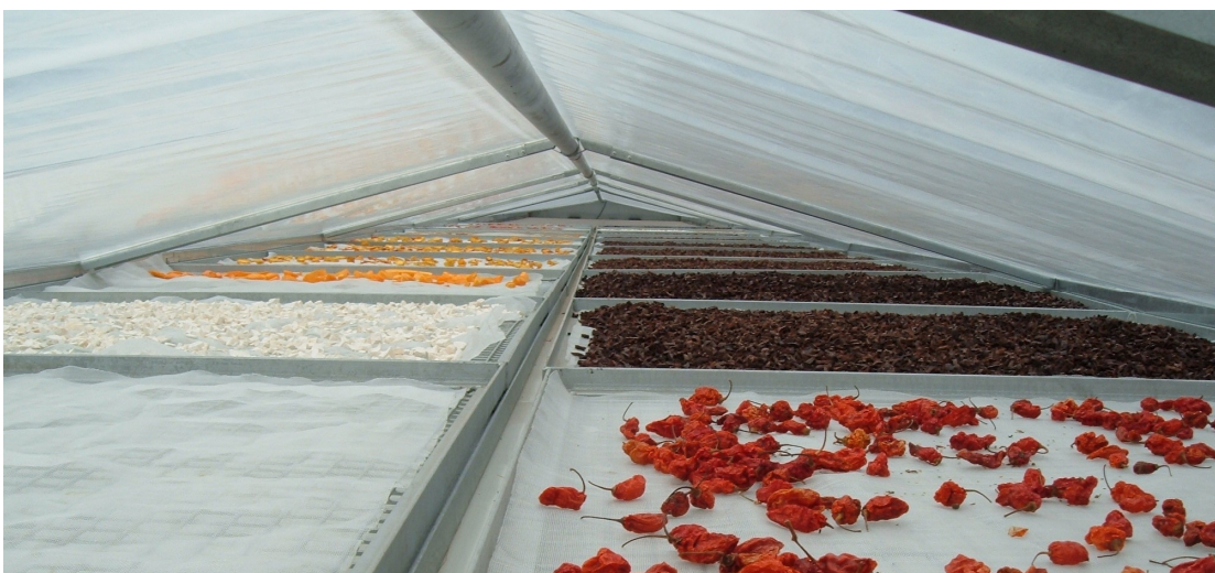
Figure 8: View inside a Hohenheim solar tunnel dryer. Photo: Tony Swetman.
