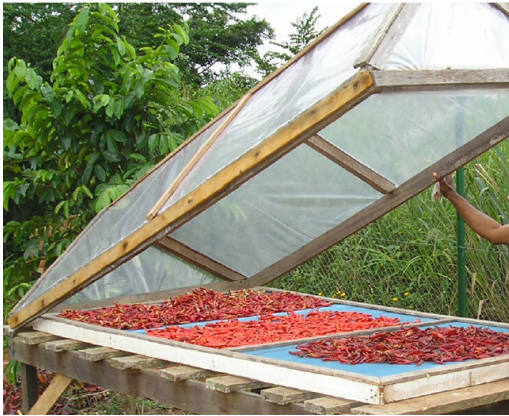
Figure 4: A small solar tent dryer, Ghana. Photo: Tony Swetman.
